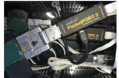
MiTM attack using Virtual Cable Mode of PP2 device
