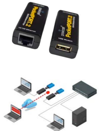
MiTM attack using Virtual Cable Mode of PP2 device
